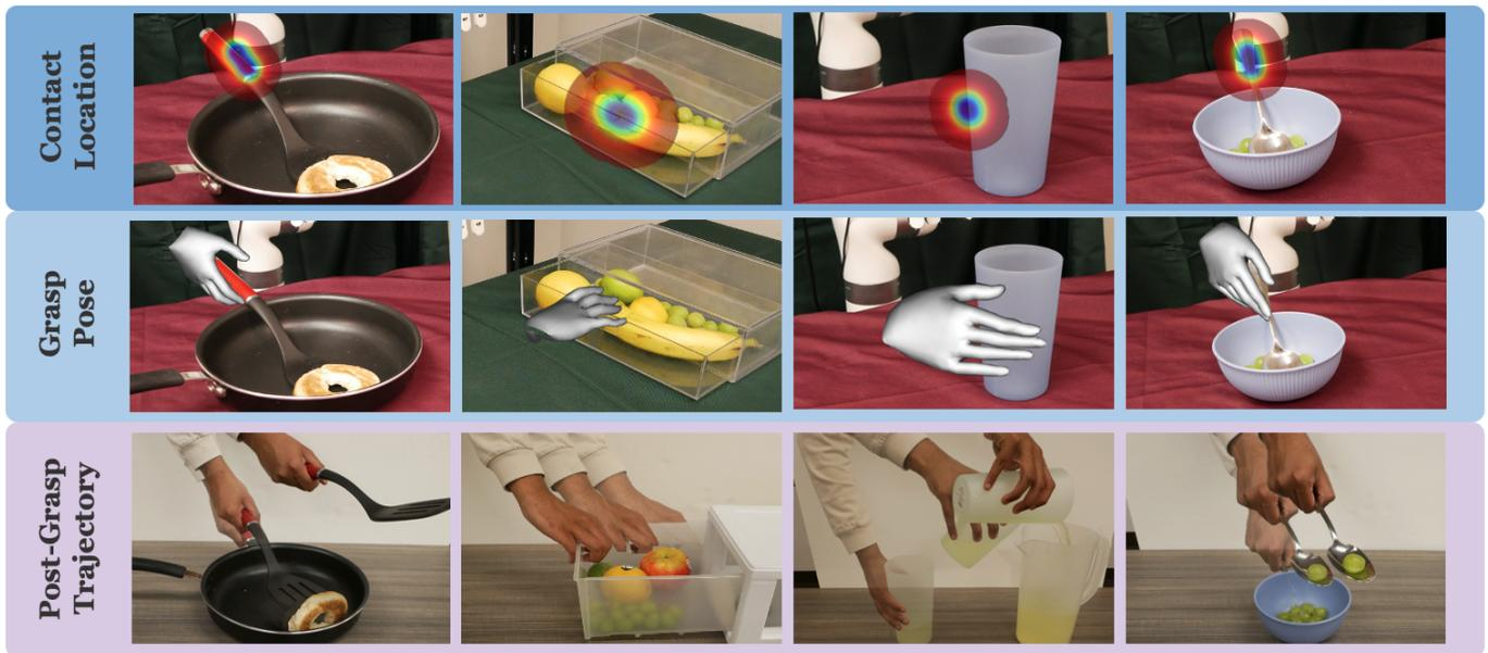
Fig. 4: We can extract different types of data from human motion. In our papers such as DEFT [3], we produce three priors from human videos: the contact location (**top row**) and grasp pose (**middle row**) from the affordance prior; the post-grasp trajectory (**bottom row**) from a human demonstration of the task.
