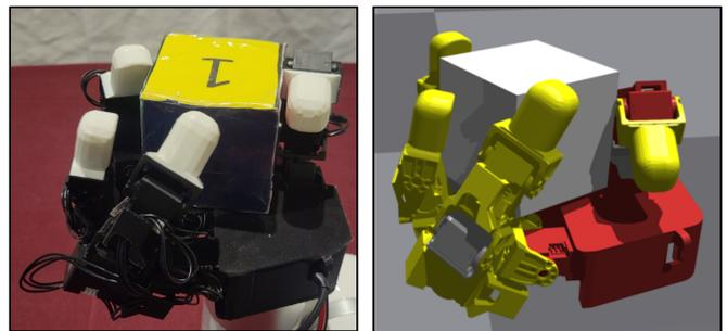
Fig. 7: **Sim2Real transfer.** *Left:* Simulated LEAP Hand in Isaac Gym [61] completing an in-Hand manipulation task. *Right:* LEAP Hand completing the same task in the real world. **This will be demoed at RSS 2024.** Please see our website <https://leaphand.com> for our open source pipeline and the paper [4] for further details.
