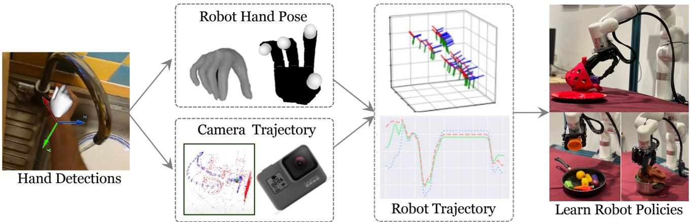
Fig. 5: To learn from human motion, we must retarget the human hand motion to the robot hand and arm. This is done in Robotic Telekinesis and Videodex by tracking the hand and wrist in the video, retargeting them using an internet-video learned retargeting method and then tracking the camera motion using SLAM. [1, 2]
