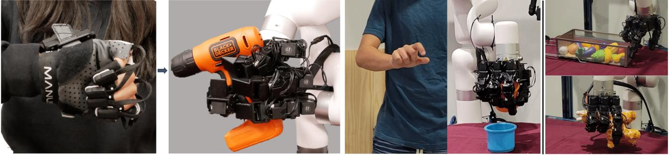
Fig. 6: We will demonstrate real robot hands doing teleoperation from VR glove and teleoperation from human video as developed in [4, 1, 6]. We will build a special version of the VR teleop system for the RSS 2024 demo that will be mobile and compatible with any arm that will be open-sourced if this demo proposal is accepted.
