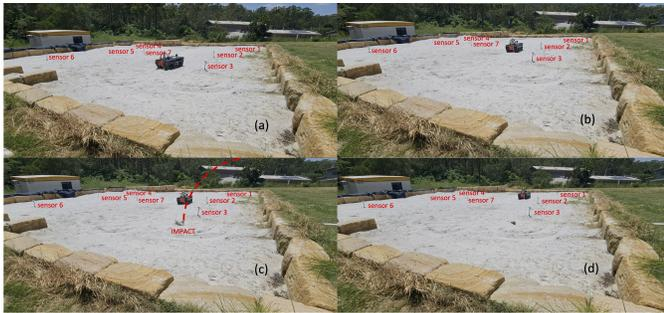
Fig. 19: The sequence of images (a-d) capture the robot position and an impact event during the 21-second mock-up demonstration: (a) robot passes by sensor 3 at  $t=7s$ , (b) robot passes by sensor 2 at  $t=12s$ , (c) a large rock is thrown in to the sandpit to demonstrate a seismic event at  $t=15.8s$ , and (d) robot passes by sensor 1 at  $t=20s$ .
