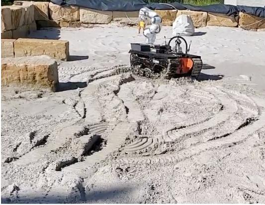
Fig. 24: Long-term robot motion causing degradation of the terrain and worsening traversability conditions at the same time making sample collection difficult in the future.
