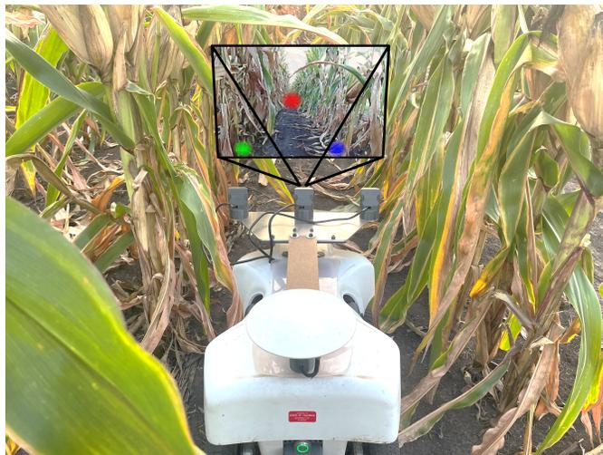
Fig. 1: CropFollow++ is a vision-based navigation system for under-canopy agricultural robots. It uses a neural network to predict the keypoints representing the crop rows from an RGB image and traverses the gap between the crop rows.
