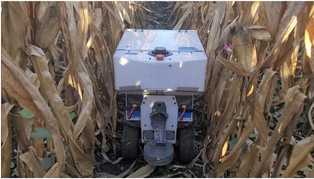
Fig. 9: CCR navigating between the crop rows. Note the minimal space available for the robot between the rows.
