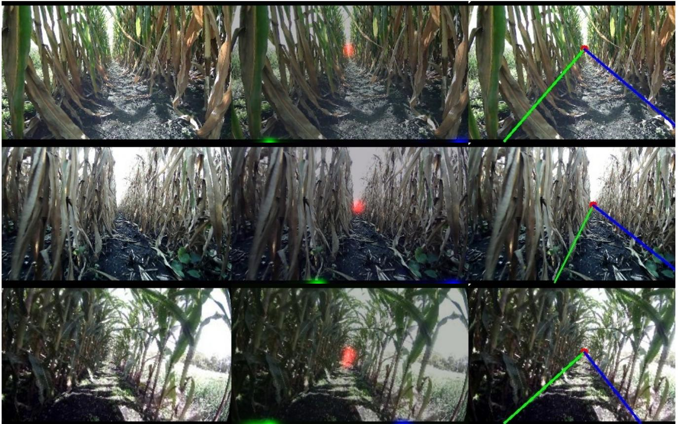
Fig. 14: **Keypoint Detection in Action:** Here we show three randomly sampled images from CCR deployment with keypoint detections. **Left:** Raw images from the CCR front camera. **Center:** Visualizations of the heatmaps for the vanishing point (red), the left point (green), and the right point (blue). **Right:** Visualizations of the keypoint outputs and the extracted vanishing lines, computed as the argmax of each heatmap.
