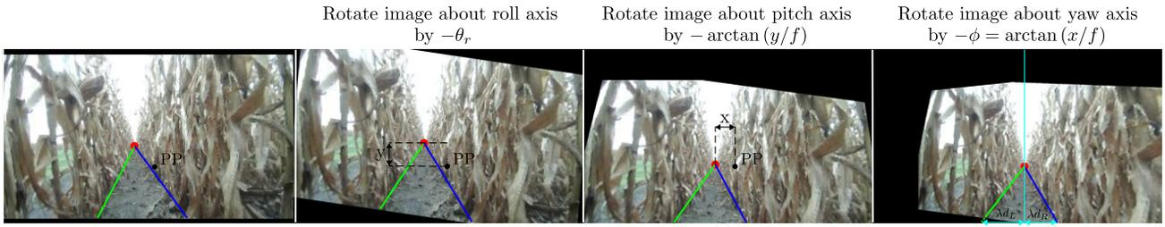
Fig. 3: Calculation of heading and distance ratio from keypoints is illustrated here. We use the roll estimation from IMU and calculate the heading angle  $\phi$  from the horizontal offset of the vanishing point from the principal point. The distance ratio is calculated from the ratio of the intercepts of the left and right crop row lines  $d_L/(d_L + d_R)$  after correcting for roll, pitch, and heading.
